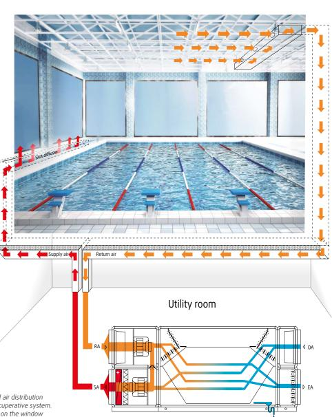
Example of an optimal air distribution system based on a recuperative system. Introduction of the air on the window facades, extraction at the top. The amount of supply and return air is constant.
