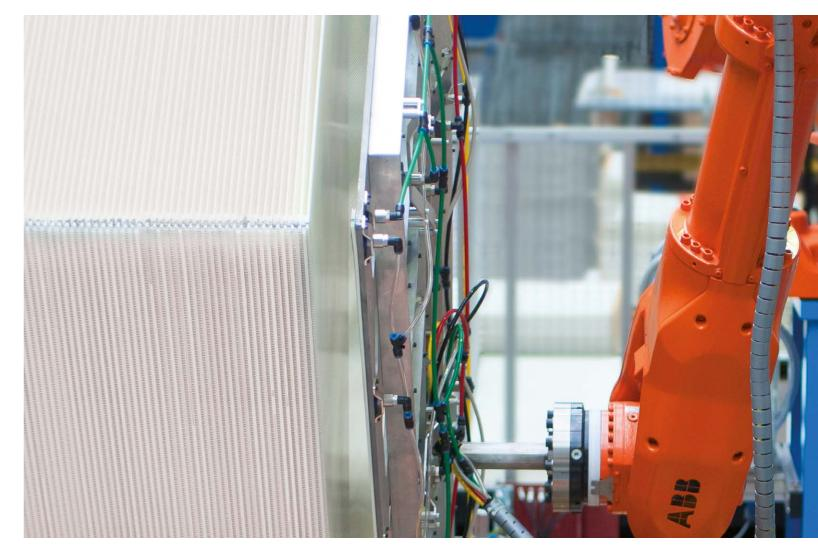
Heat exchanger made of polypropylene, fully automated production.
