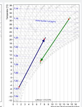
the design if the dew point is not reached, since the condensate produced by a heat wheel gets into the outside air flow with the help of the rotation. This moisture recovery increases the absolute water content in the supply air and has to be compensated for with a greater quantity of outside air. The significantly higher fan input power results in higher energy requirements in addition to the driving power of the heat wheel.
